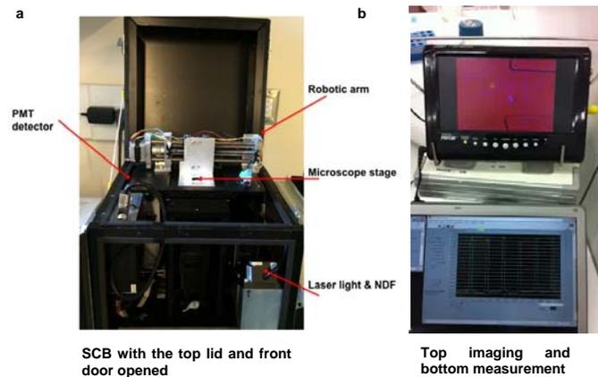
**Fig. 1. Single cell bioanalyzer (SCB) shown in (a) and the associated TV monitor for optical imaging of the prostate cancer cell and the computer screen for fluorescent measurement of 6 peaks above background shown in (b).**
