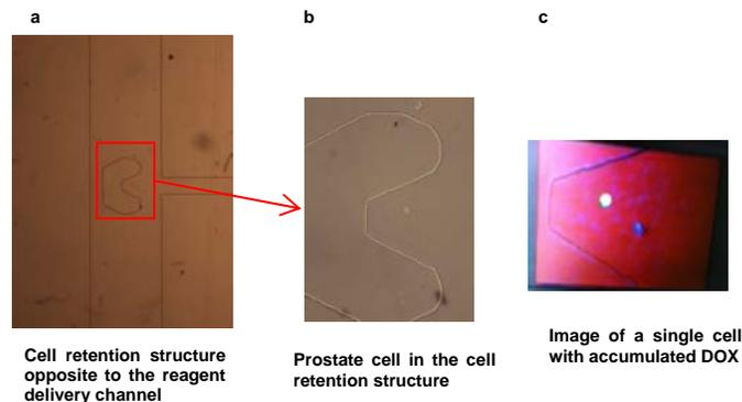
**Fig. 3. Cell retention in a microfluidic biochip.** (a) The cell retention structure is located in the chip to retain cells. (b) Closeup of a prostate cancer cell retained in the cell retention structure. (c) Optical imaging (under red light) of a single PC-3 RX-DT2R cell with fluorescent emission in yellow due to DOX accumulation.
