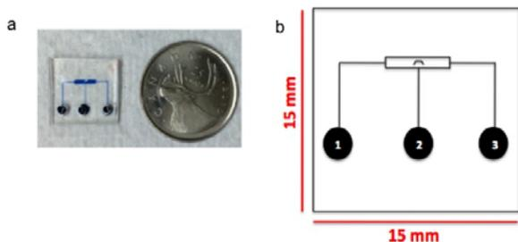
**Fig. 2. The microfluidic chip.** (a) Image of the microchip (1.5 cm × 1.5 cm) filled with a blue food dye. A Canadian quarter (25 cents) was placed next to the chip for size comparison. (b) The schematic showing reservoir 2 used for drug delivery; whereas reservoirs 1 and 3 served as the cell inlet and waste, respectively.
